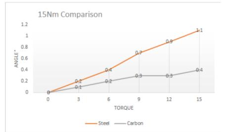
· Test results and comparison of 300Nm wrenches:
