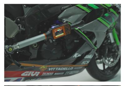
Alert management / Auto diagnostic: Transducer Alert : Offset comparison Gyroscope Alert : Stability of 0 speed Over torque Max value Over torque List of last 16 over torque & When happen Maintenance counter with the Alarm number
