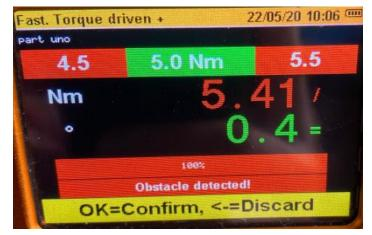
On LAB/SPC : The obstacle detection function is always active without possibility to disable it
